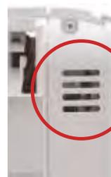
Sensor for indoor temperature and humidity
